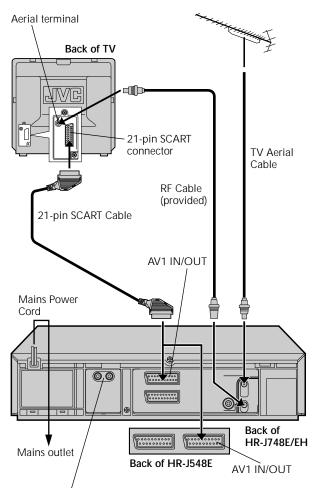
AUDIO OUT(put) connectors (HR-J748E/EH only) For connection to the audio input connctors on a Hi-Fi stereo system It's essential that your video recorder be properly connected. Follow these steps carefully. THESE STEPS MUST BE COMPLETED BEFORE ANY VIDEO OPERATION CAN BE PERFORMED.
